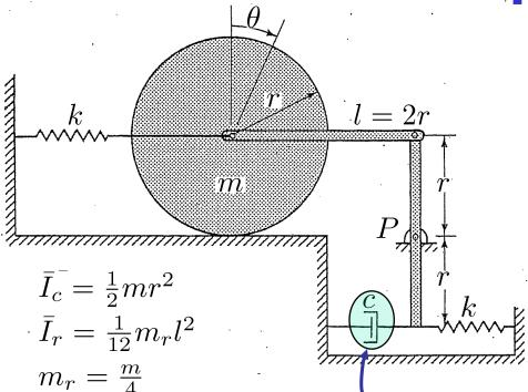
Use  $T_{max} = U_{max}$  to determine <u>undamped</u> natural frequency  $\omega_n$  for the system
