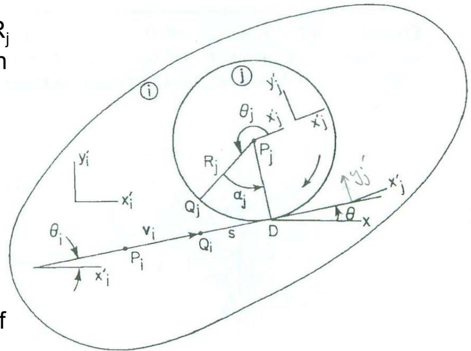
Figure 3.4.5 Rack and pinion.
