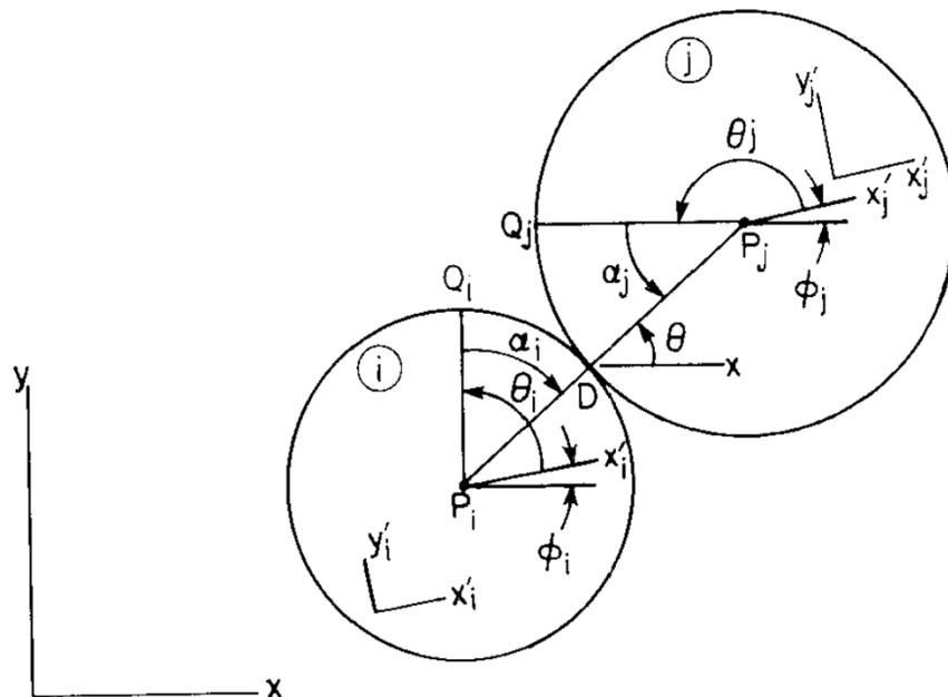
Figure 3.4.2 Geometry of gear set.
