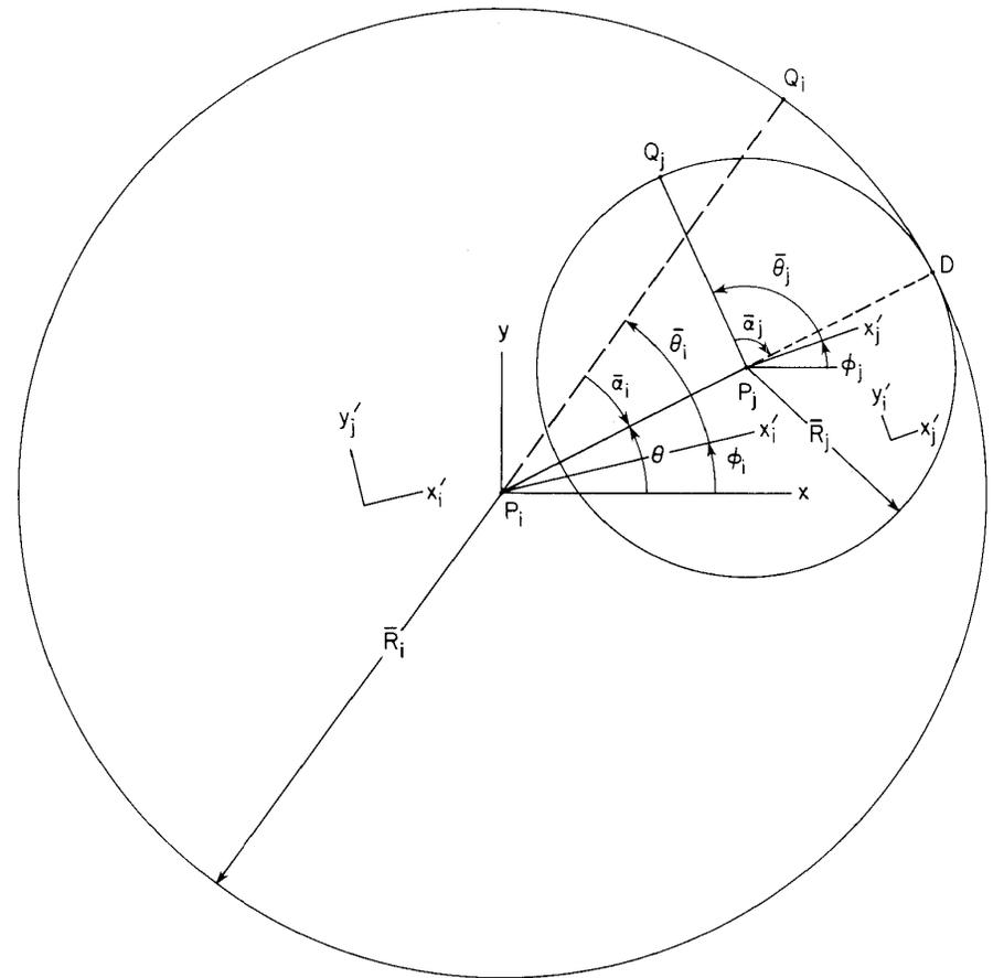
Figure 3.4.4 Concave-convex gear set.
