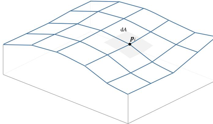
Figure 5: The original SCM soil, based on uniform structured grids.
