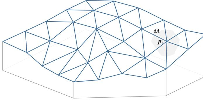
Figure 6: The modified SCM soil, based on unstructured triangular grids.
