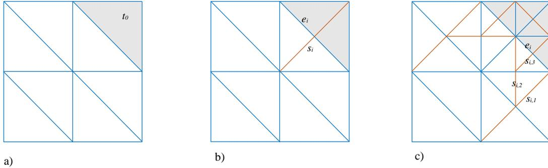
Figure 8: The LEPP algorithm for mesh refinement.
