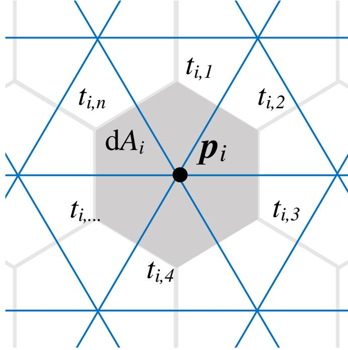
Figure 7: The  $i$ -th weight for quadrature of pressure integral (in case of regular triangle grids).
