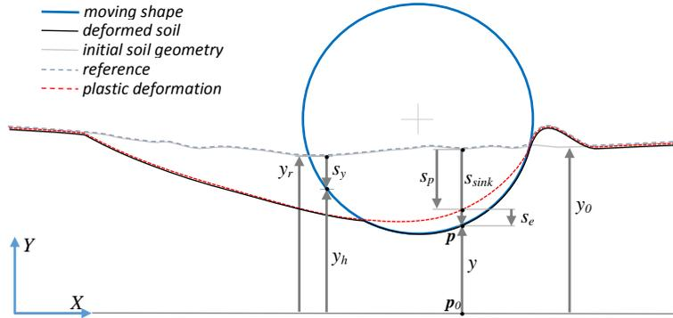
Figure 2: Deformation of the soil: variables used in formulas.
