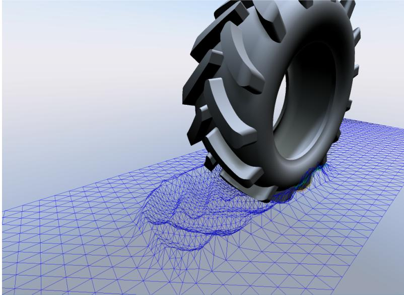
Figure 9: Automatic mesh refinement under the wheel footprint and in the surrounding region.
