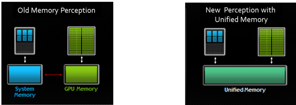
Figure 2. Prior to CUDA 6, there was a clear physical and logical separation between the host and device memories. UVA blurred the logical separation while UM went one step further. The elimination of the physical separation has already taken place on NVIDIA’s Tegra K1 SoC architecture.
