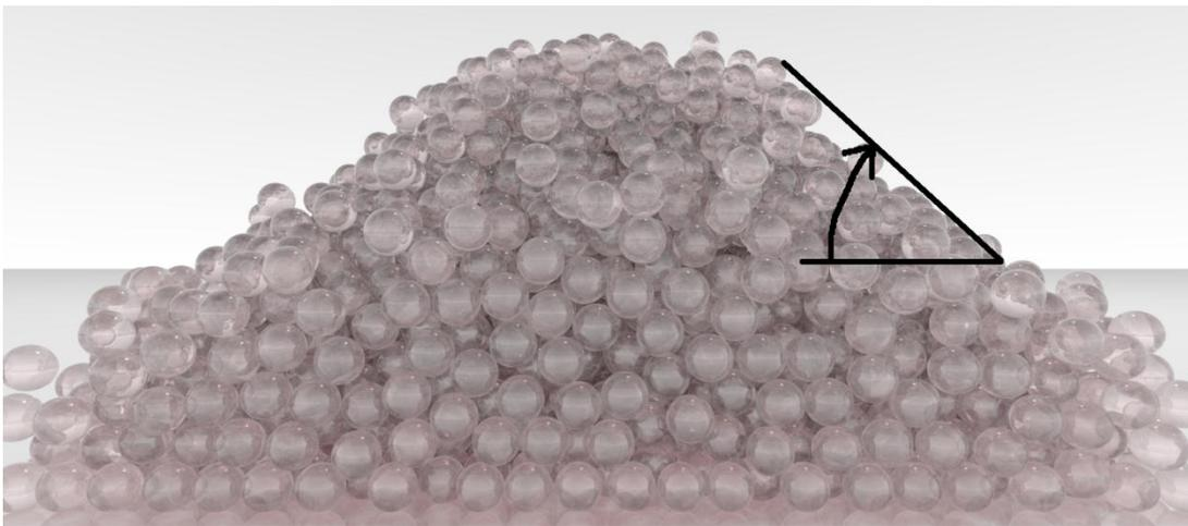
Figure 5: Measuring the angle of repose for the simulation with nominal friction coefficient of 0.90
