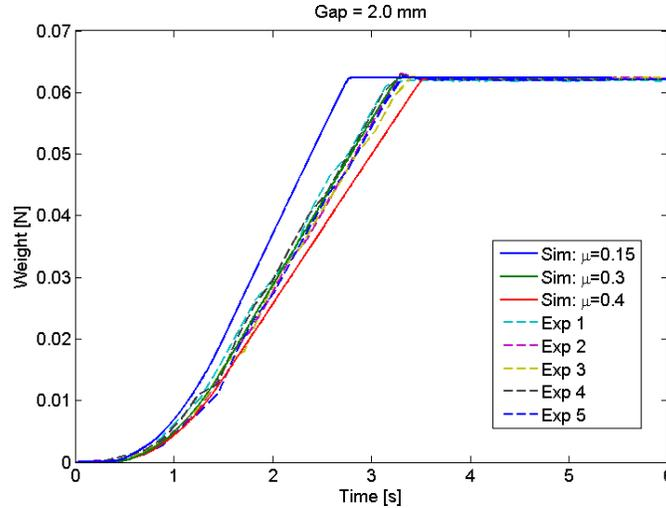
Figure 8: Experimental and simulated mass flow rate data for a gap opening of 2.0 mm
