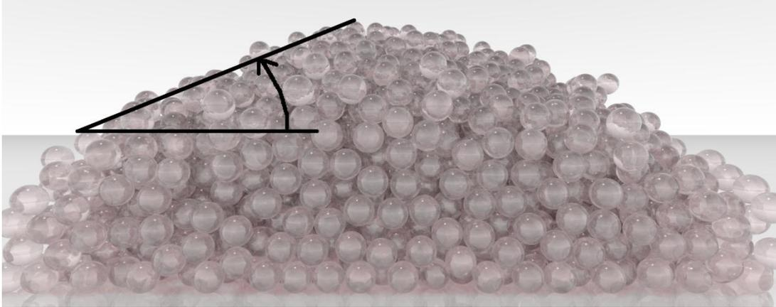
Figure 4: Measuring the angle of repose for the simulation with nominal friction coefficient of 0.40
