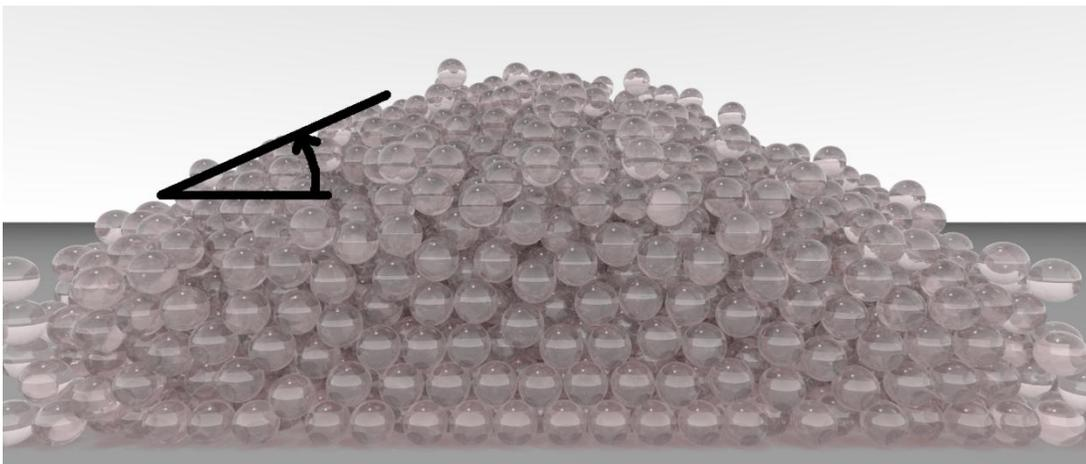
Figure 2: Determining the angle of repose of glass beads by simulation
