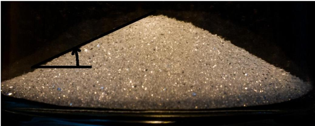
Figure 1: Experimentally determining the angle of repose of glass beads
