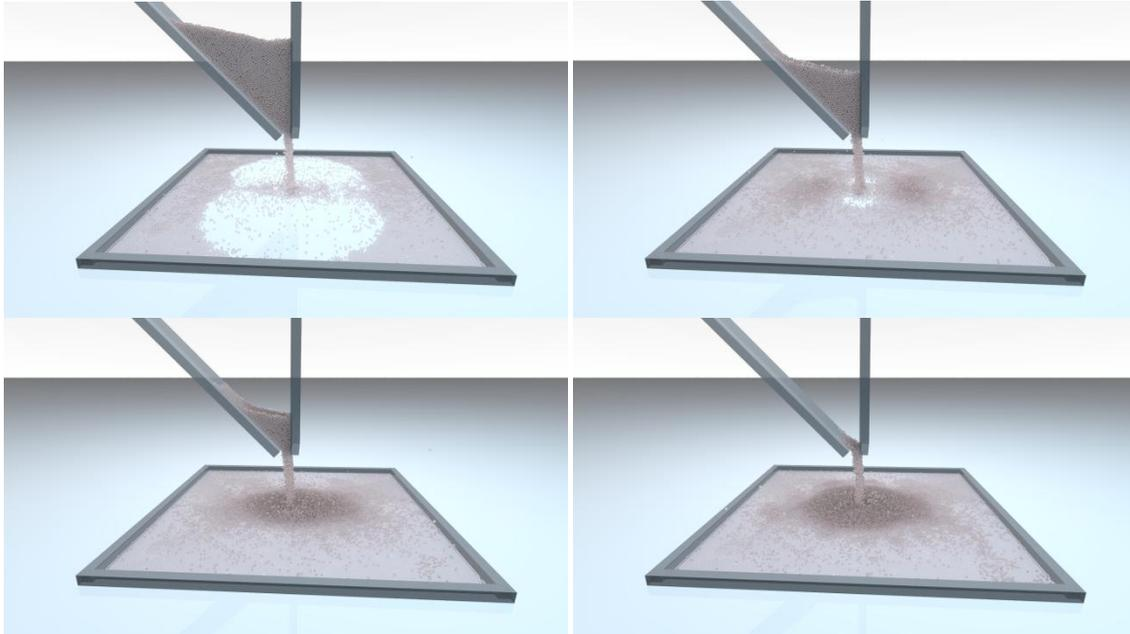
**Figure 7: Renderings of four time steps in a simulation of granular material slit flow**
