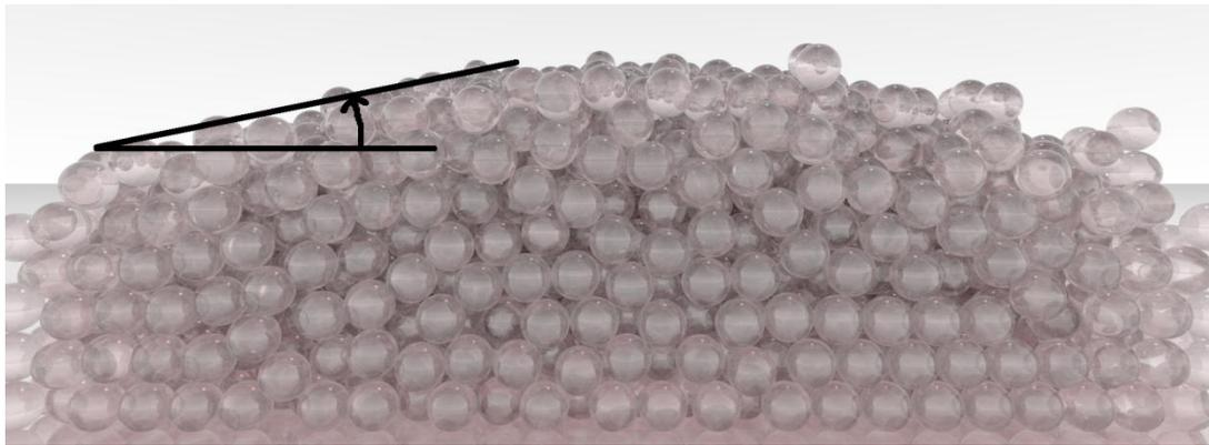
**Figure 3: Measuring the angle of repose for the simulation with nominal friction coefficient of 0.20**
