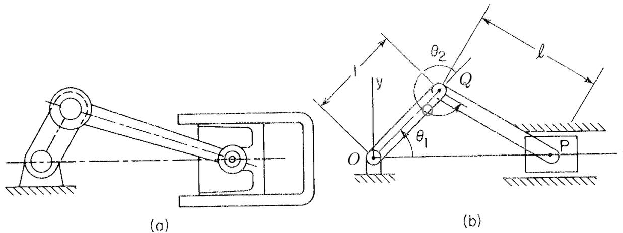
**Figure 2.4.6** Slider-crank mechanism. (a) Physical system.
