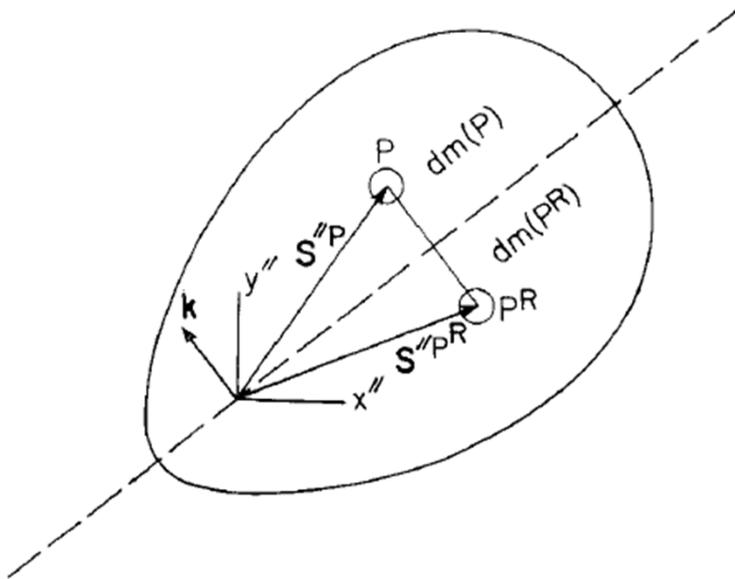
Figure 6.1.4 Body with axis of symmetry.
