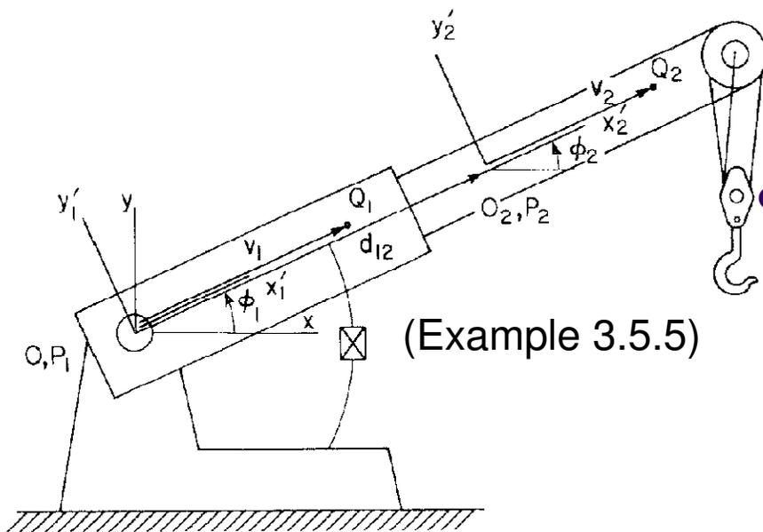
**Figure 3.5.10** Wrecker boom with a translational-distance driver.
