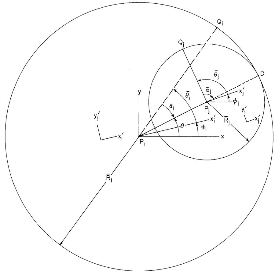
Figure 3.4.4 Concave-convex gear set.
