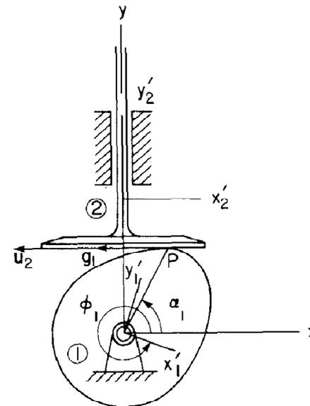
Figure 3.4.11 Cam-flat-faced follower in an internal combustion engine.
