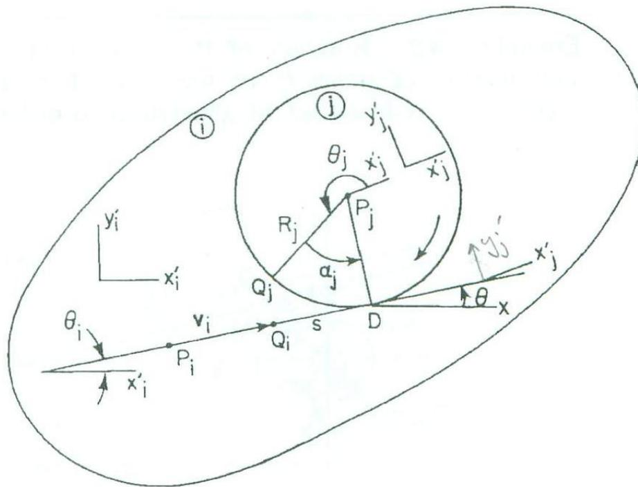
Figure 3.4.5 Rack and pinion.
