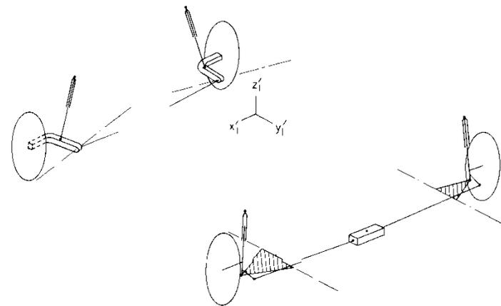
Schematic of car suspension
